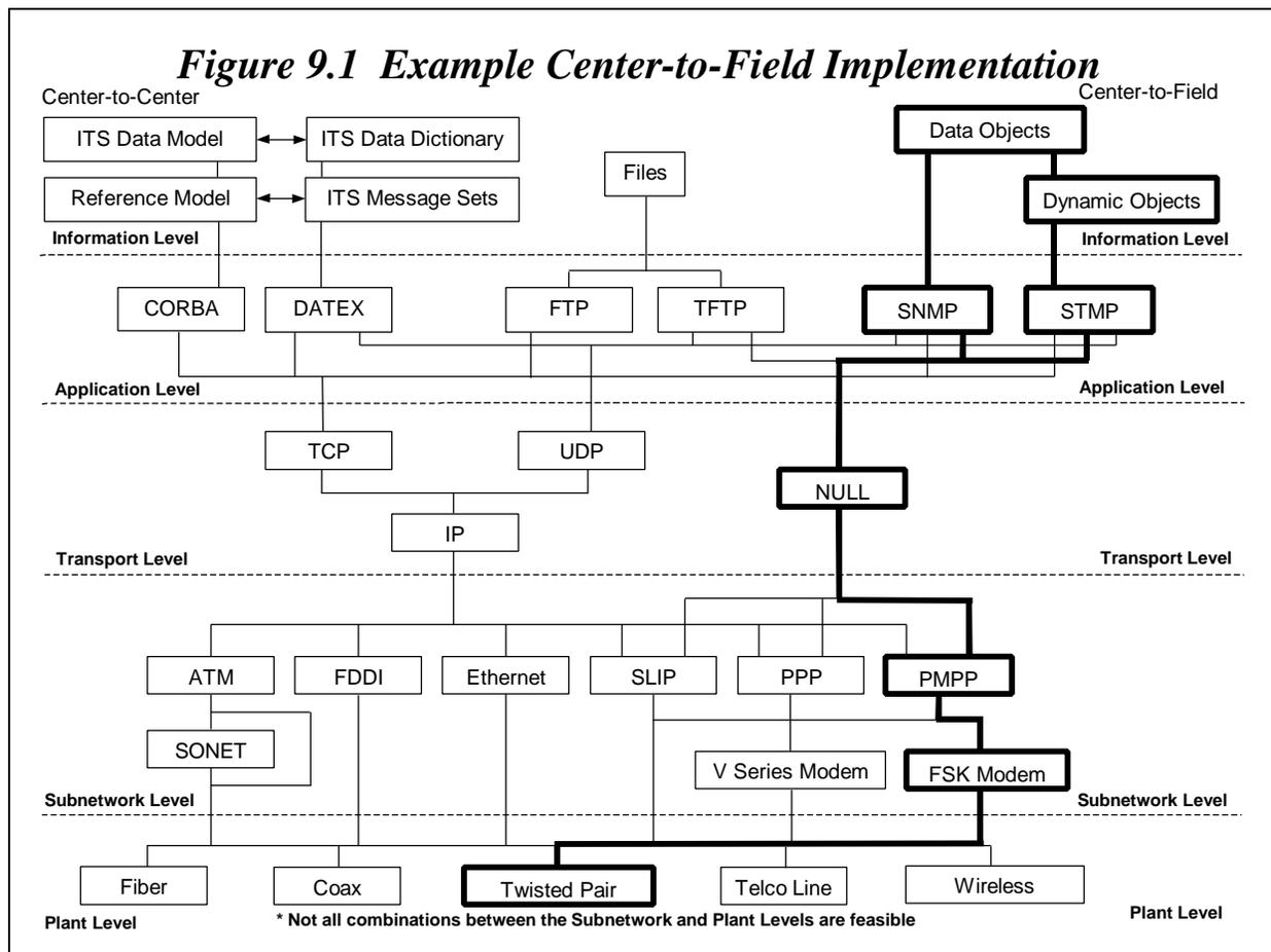
The Subnetwork Level standard selected in this example is Point to Multi-Point, FSK modems. The Plant Level in this example NTCIP implementation is shown to be agency owned twisted pair wire, but any suitable media can be used.
