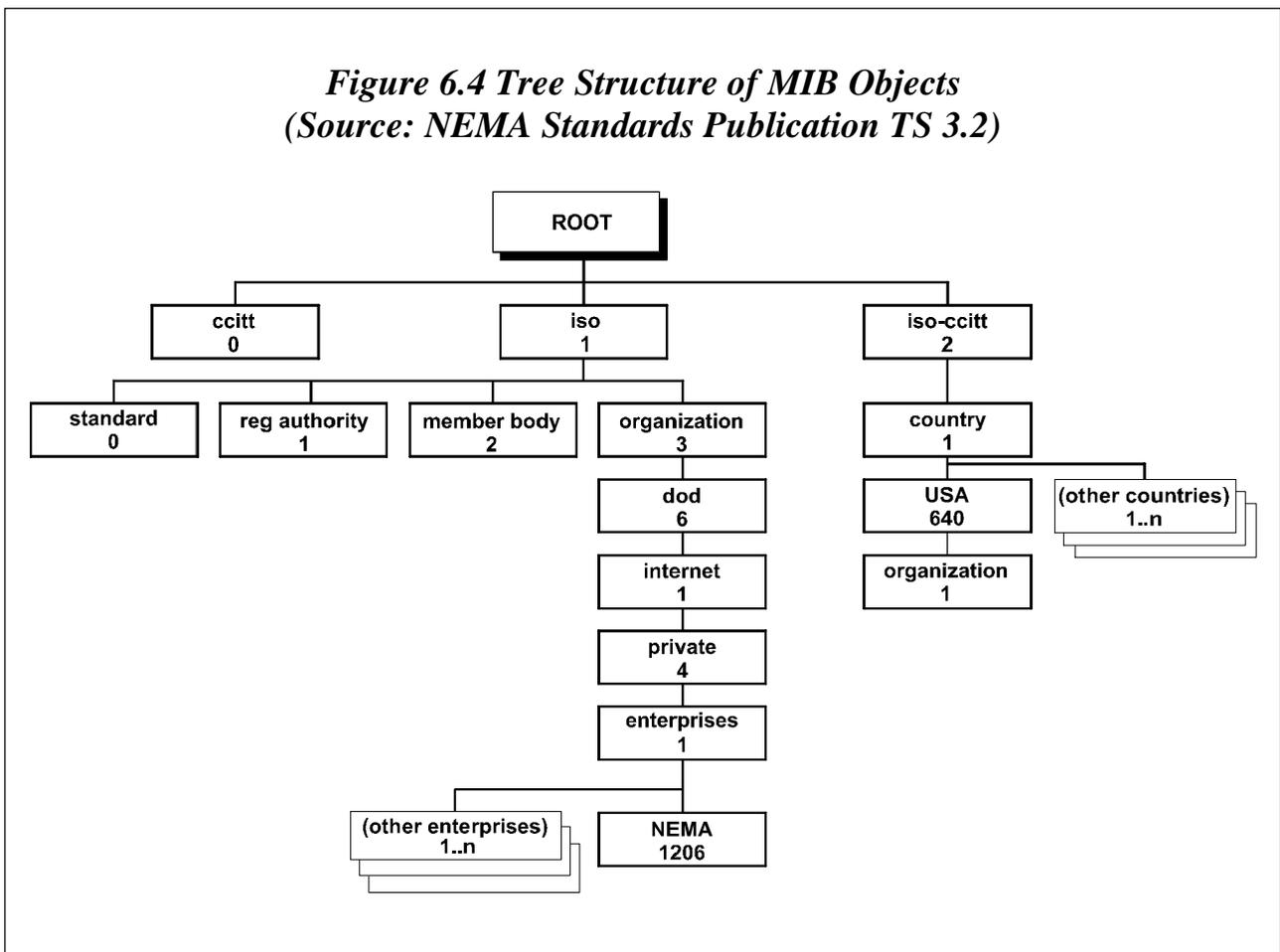
The MIB objects are related by device type (e.g., a traffic controller MIB or a message sign MIB). These device MIBs are called modules. NTCIP has MIB modules for actuated traffic
