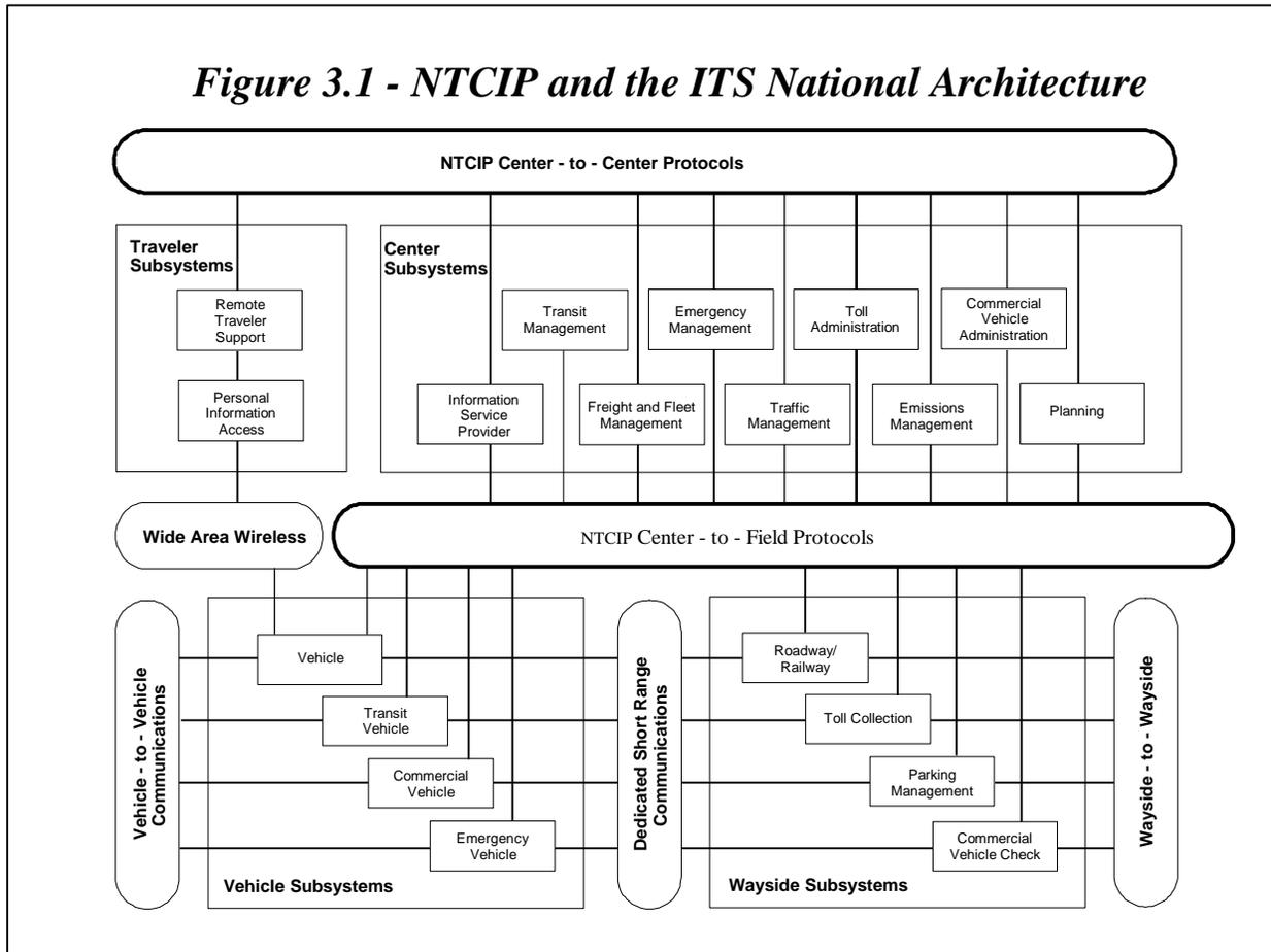
The following are examples of systems and devices that can take advantage of NTCIP:
