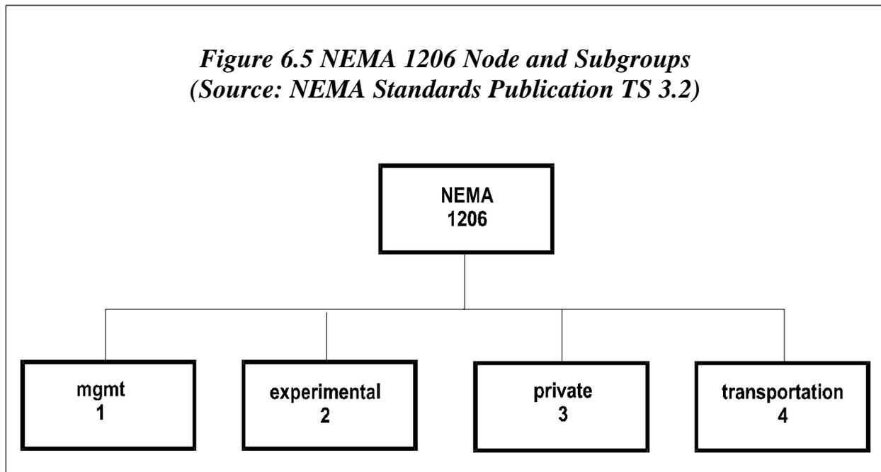
Everything below the transportation node constitutes the TMIB. Within the TMIB there are protocol, device, and tcip object groups. The device group has subtrees for each of the supported devices: asc, ramp meter, dms, cctv, ess, global, etc. Branches are added as new devices are included in NTCIP.
