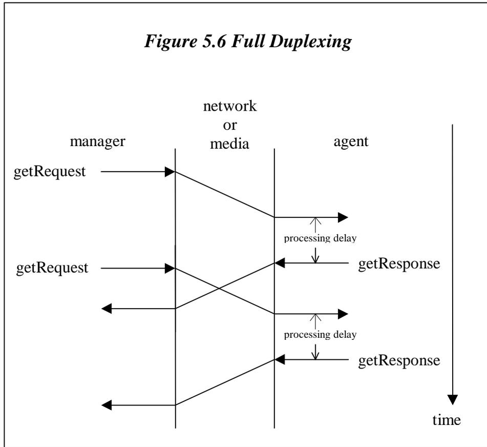
The duplexing mode of operation can have a significant impact on timing. In full-duplex mode, commands and responses can overlap. A second command can be sent while the response to a previous one is being received. In half-duplex mode, a second command can not be sent until the response to the first is received. Full-duplexing can effectively cut the data rate requirements significantly. The following summarizes the delays that will be used in what follows.
