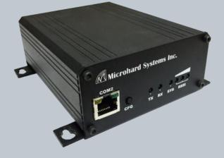
A complete wireless solution for integrating industrial Ethernet and serial devices into IP/Ethernet networks. The IP921 allows Ethernet devices to share high speed wireless media and provides a wireless gateway for network applications to access serial devices. The IP921 also features flexible maintenance utilities and network management facilities.
