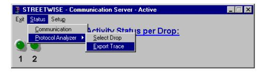
The Protocol Analyzer provides the ability to capture and trace all NTCIP data between StreetWise and the field devices. The trace capture is a byte-by-byte definition of the protocol transmitted (TX) and received (RX) from the field. These byte definitions agree with the byte definitions required by the NTCIP objects in the NEMA protocol.
