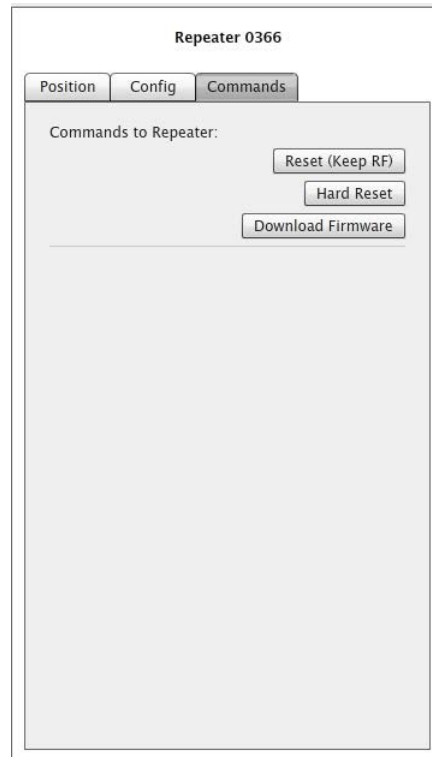
Figure 5.35. Repeater Configuration window (Commands tab)
