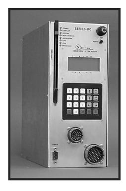
The **Trafficware Model NM512-E123NEMA Conflict Monitor** is an enhanced keyboard-programmable conflict and power monitor that exceeds NEMA TS1 specifications. User interface is simplified by an LCD display and menu-driven software.
