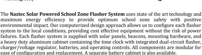
Flasher systems may be manually operated or programmed via the real-time-clock keyboard. The **Chronomax** time clock may also be operated or programmed remotely via special PC-based software and a built-in pager or radio. Non-wireless communications configurations such as fiber optic or twisted pair are also available. With these communications options, the school zone flasher system can be easily integrated into an advanced traffic management system.
