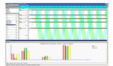
**Time-Space Diagram** – The user can plot a real-time timespace diagram by selecting a group of controllers. The resulting diagram shows split times, offset times, bandwidth values, speed, and other enhancements. The split data used
